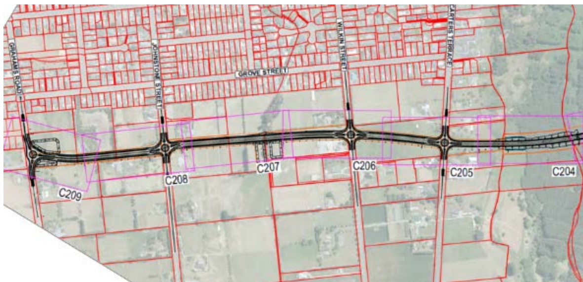
Figure 2-2 - Section of Proposed Road Through Existing Rural Land South of Tinwald
