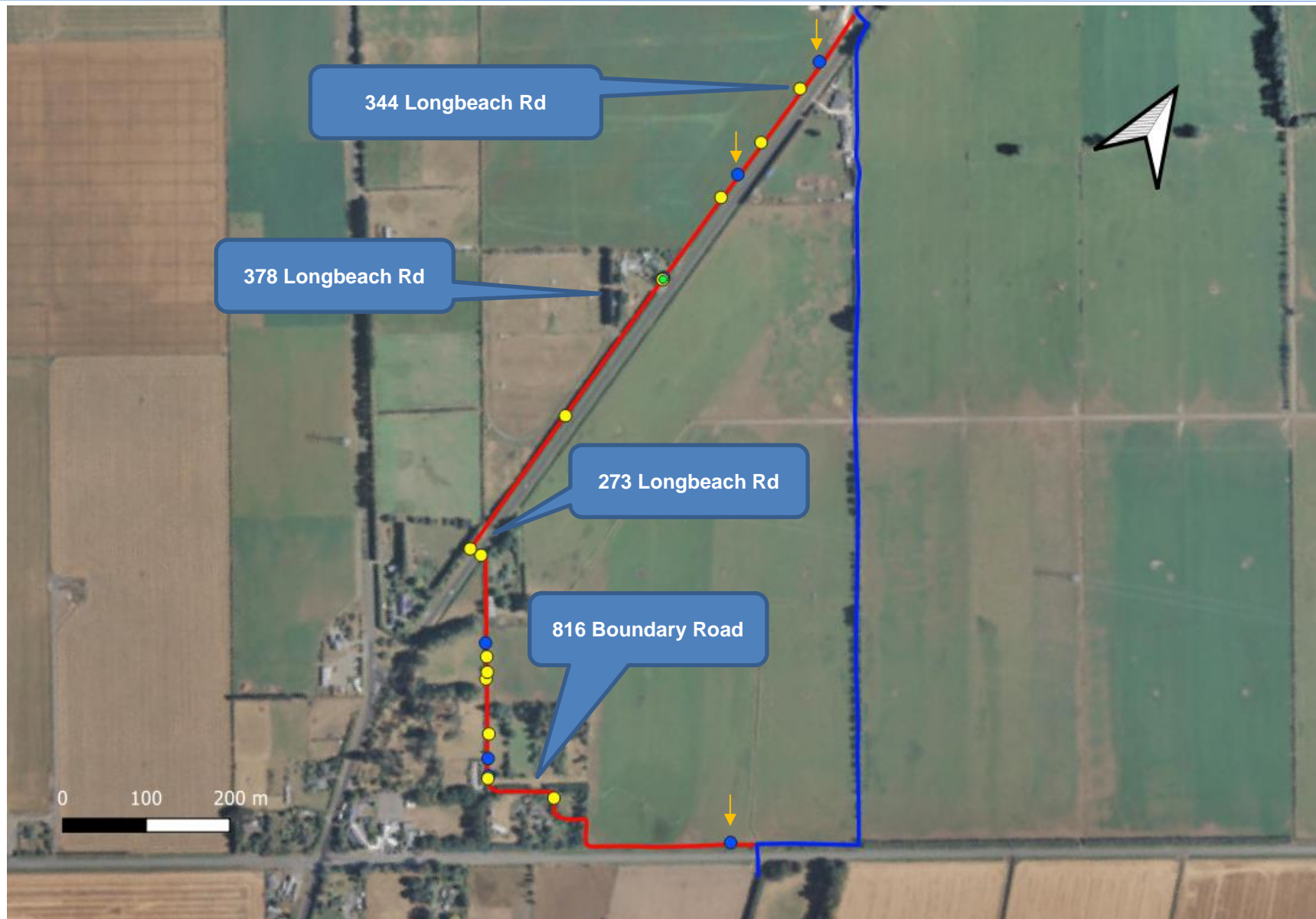
Figure 1. Showing the current path of the Willowby Water Race (red line), and the alternative water race route (blue line). Areas surveyed using GM traps are marked in blue, electric fishing sites are marked in yellow, and the site of invertebrate sample is marked in green. Orange arrows mark the sites where upland bullies were identified.
