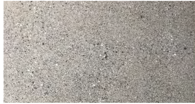
Exposed aggregate concrete - author
