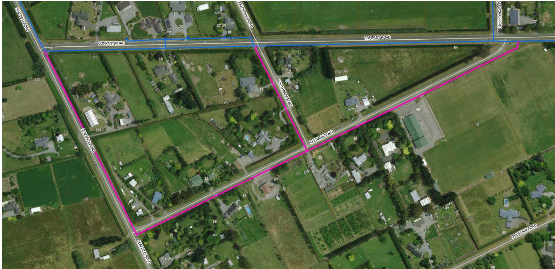
Plan showing the proposed pipe route in purple, and existing network in blue
