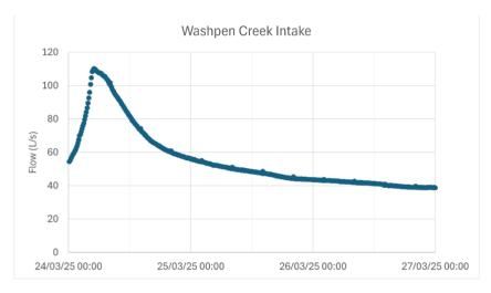
Figure 5. Flow at Washpen Creek Intake.
