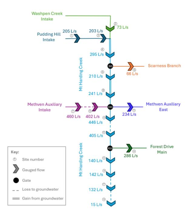
Figure 2. Flow gauging schematic diagram of the Mt Harding Creek network (SG = Scarness Gate, DG = Draytons Gate, and FDG = Forest Drive Gate).
