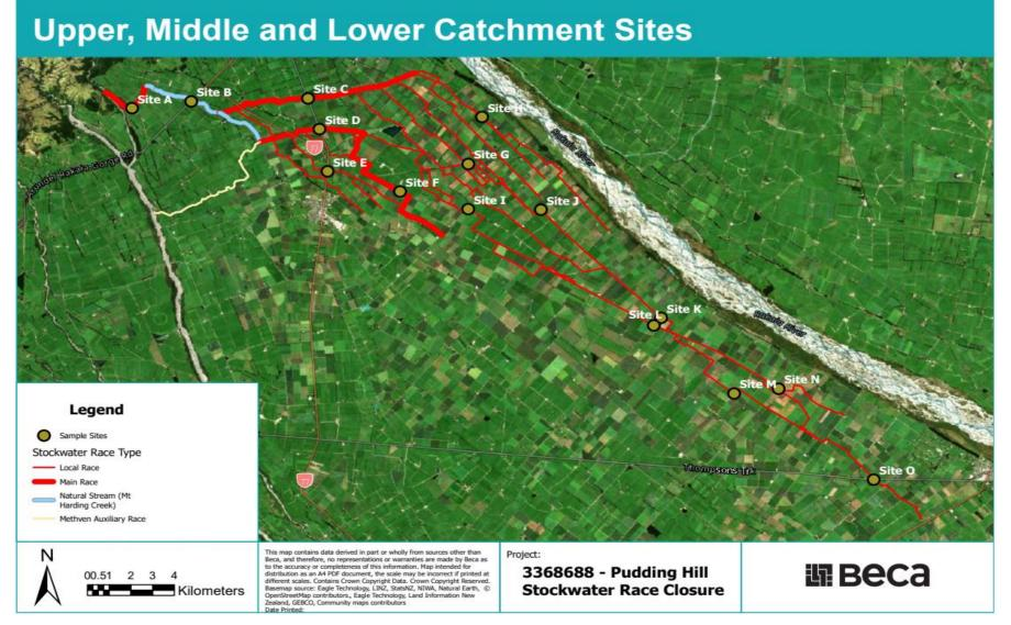
**Figure 1**. Site map of the Pudding Hill stockwater race network including the sample sites assessed in this investigation, the extent of the race network under assessment, the sections of the race network that are classified as a natural stream, main race or local race and the connection to the Methven Auxiliary race. Note: The Methven Auxiliary race is not within the scope of this assessment as it is not proposed to be impacted by the potential closure of the Pudding Hill network.
