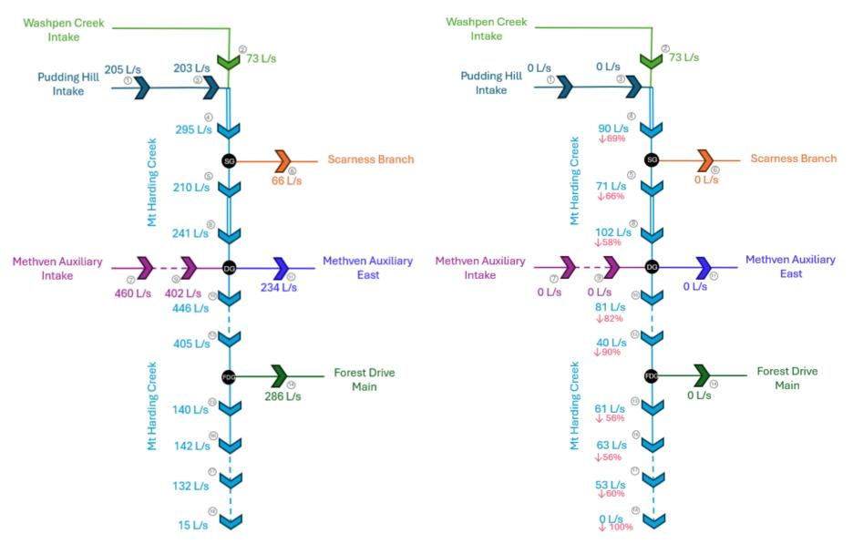
Figure 3. Measured flow gauging scematic (left) and modelled flow of the Mt Harding Creek Network under the post-closure scenario (right).
