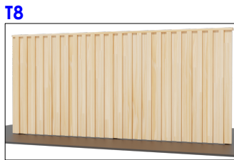
1.8m High timber board and batten fence with capping. Battens to face the street/JOAL*
