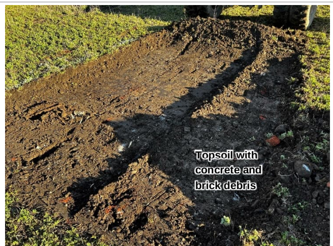
Photograph 7. View of TP11 showing topsoil with included debris
