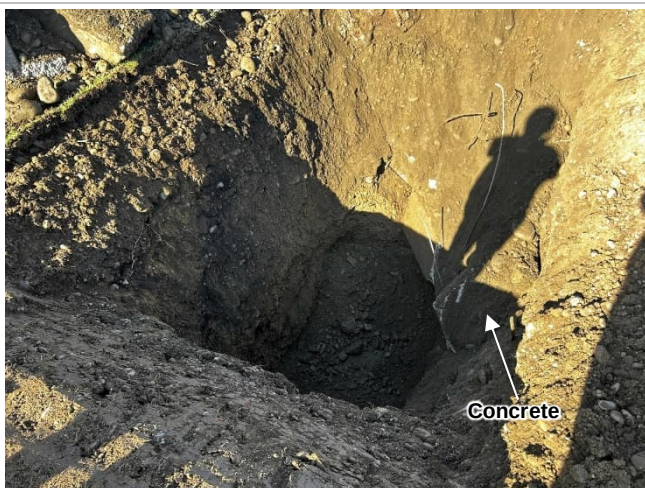
Photograph 10. View of TP12 showing reinforced concrete
