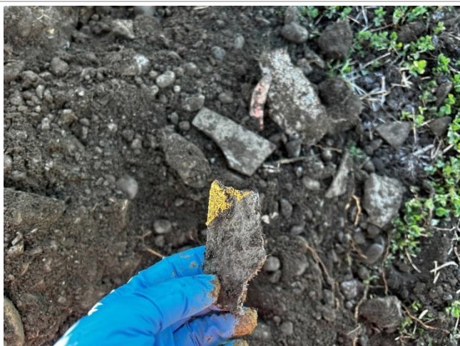
Photograph 8. View of ACM fragments encountered at TP9
