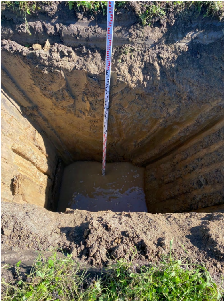
Photo – Soakage Test Pit 9
