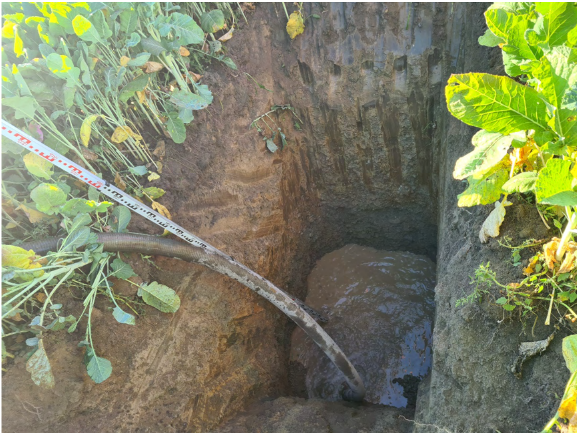
Photo – Soakage Test Pit 6
