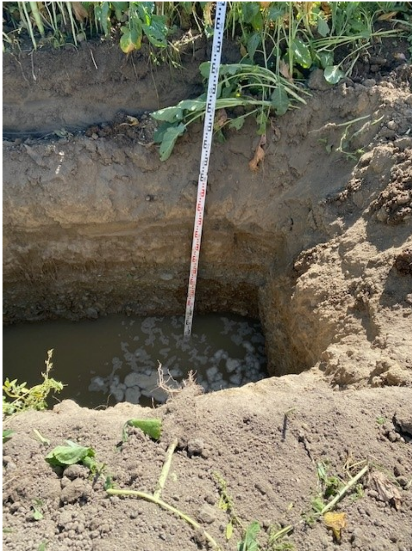
Photo – Soakage Test Pit 5
