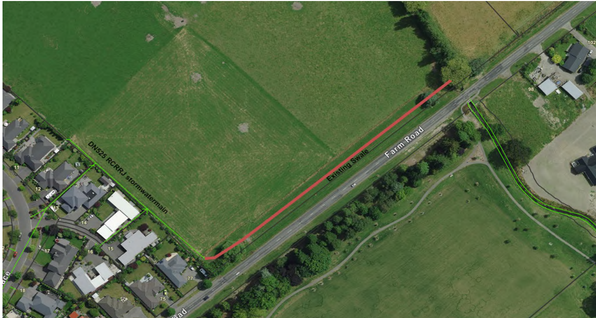
Figure 20: Existing DN525 Pipe (Green line) and Swale (Red line)
