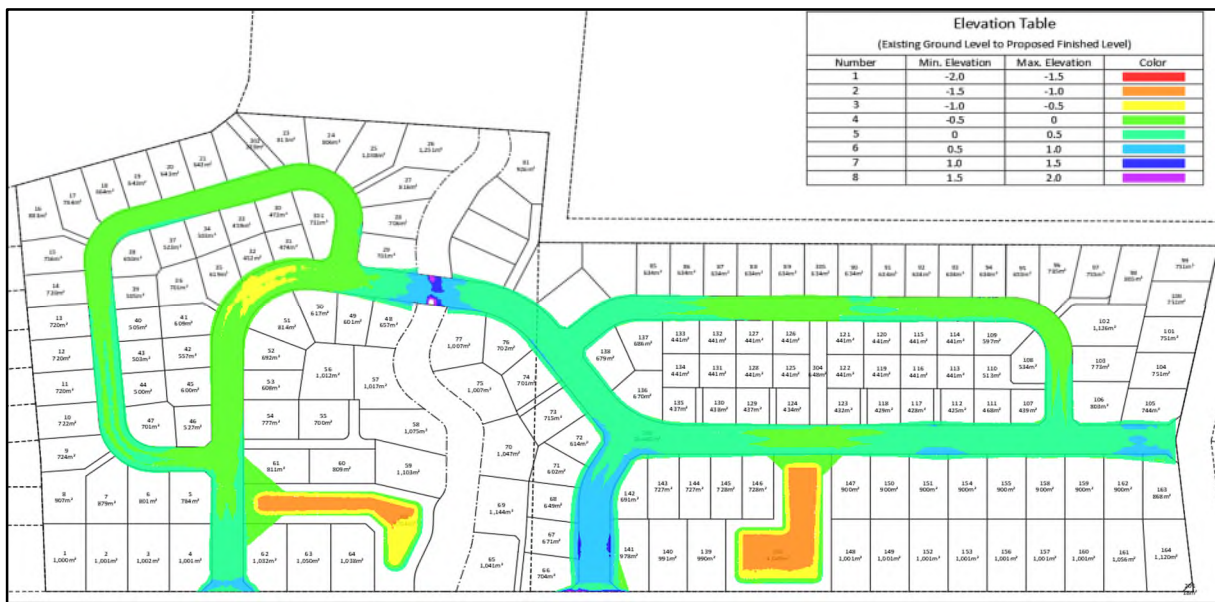
Figure 6: Excavation (Cut and Fill) Heat Map
