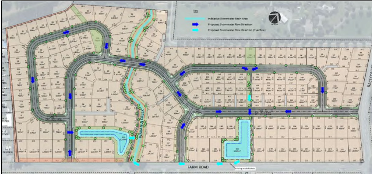
Figure 25: Stormwater Secondary Flow Path
