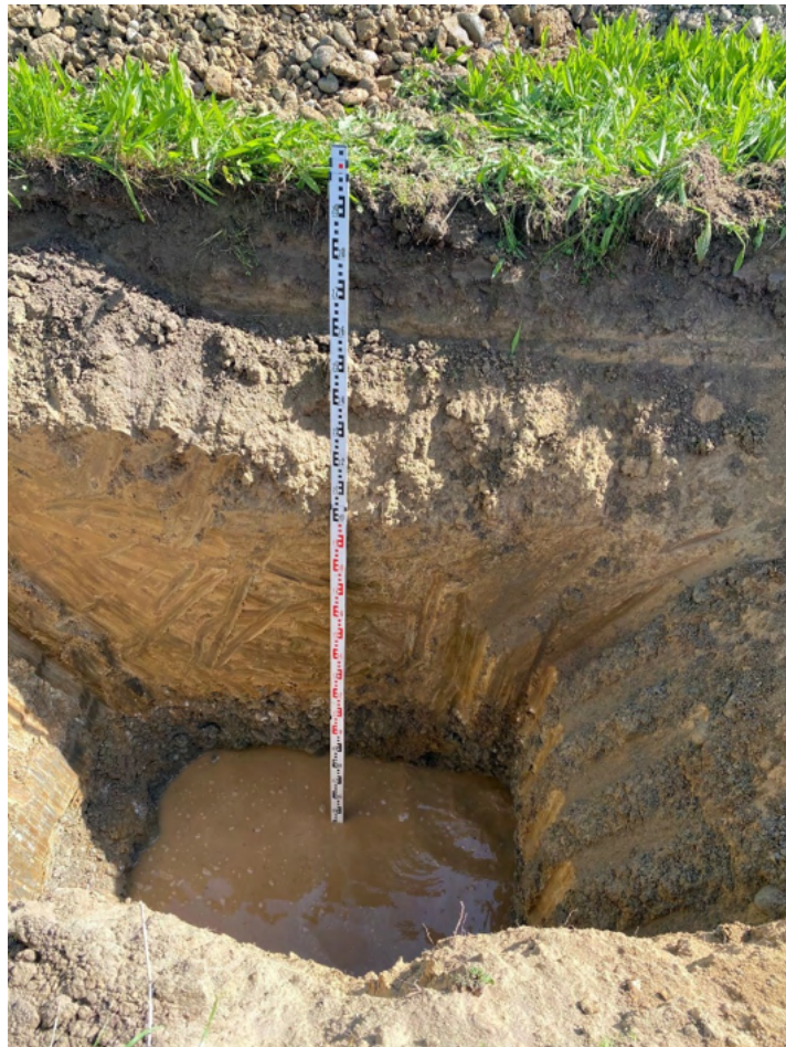
Photo – Soakage Test Pit 3
