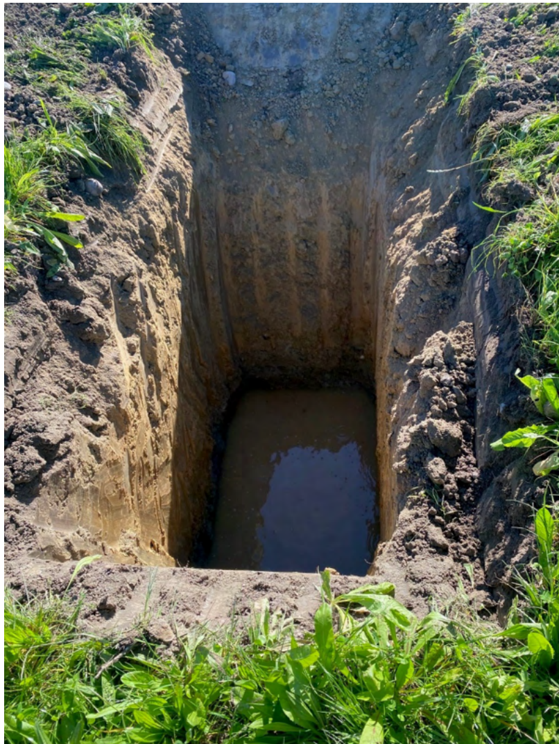
Photo – Soakage Test Pit 7
