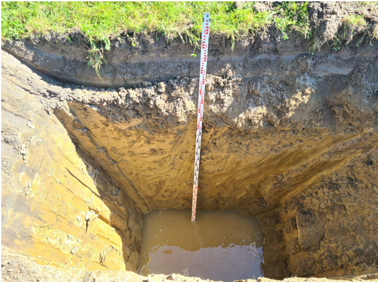
Photo – Soakage Test Pit 8
