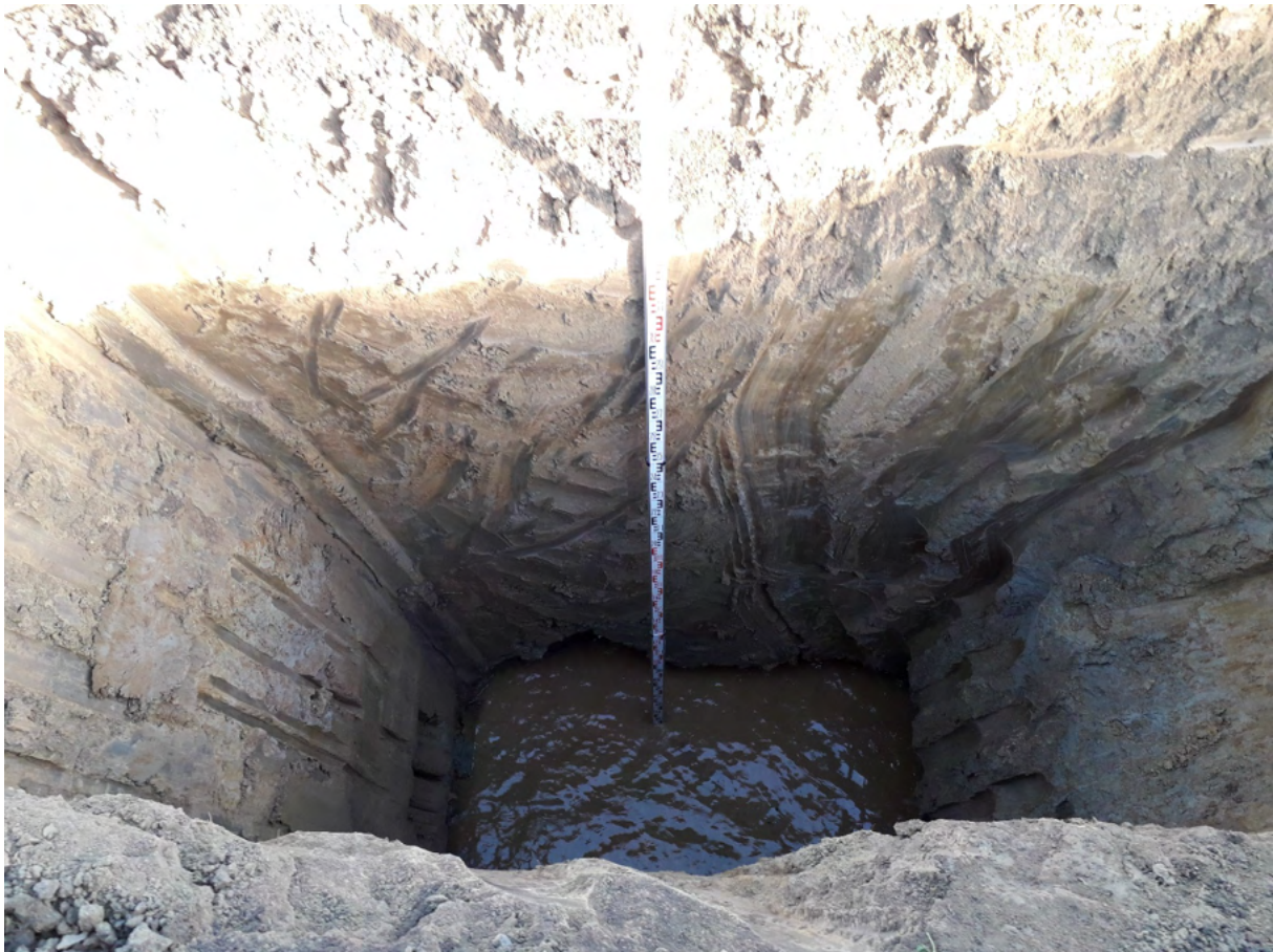
Photo – Soakage Test Pit 1
