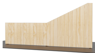
1.0 -1.8m High timber paling driveway visibility fence. 1m length panel to extend atleast 2m in length. Confirm on site. *
