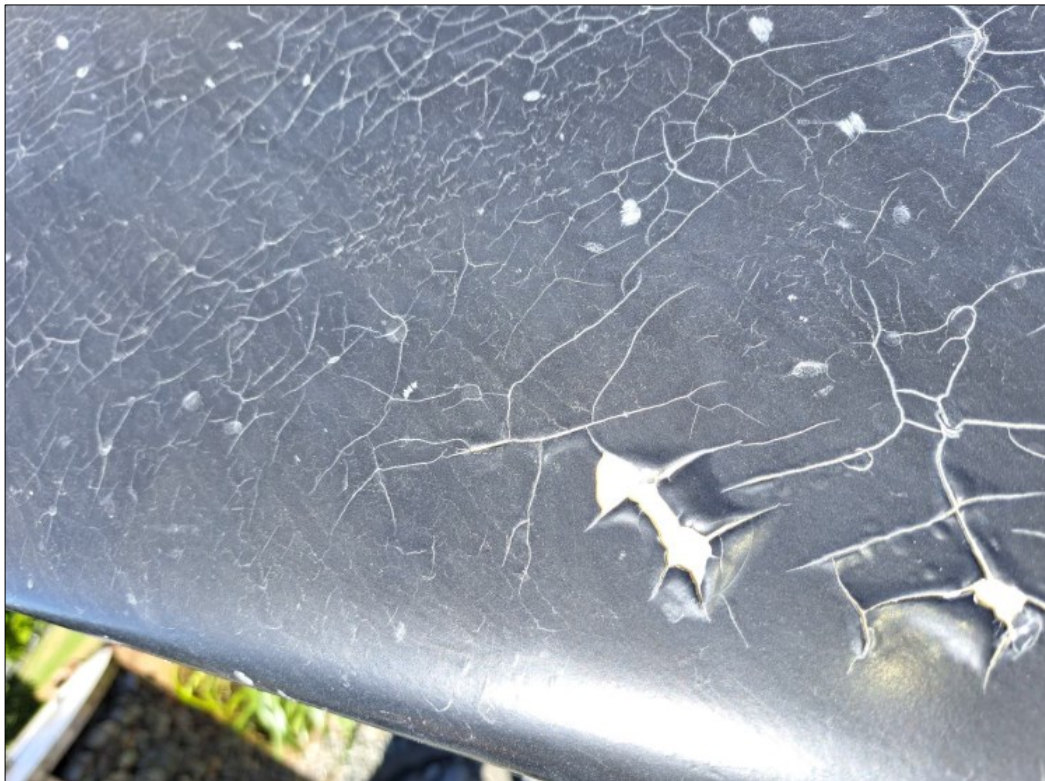
Figure 2 – Close up view of cracking and crazing on top of the salmon tail
