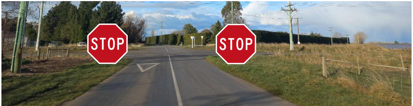
Junction Rd / Coldstream Rd (West Approach) – Change to Stop Control. Upgrade to large 1200mm stop signs and white background 200mm stop ahead (gated). Average visibility to the right.
