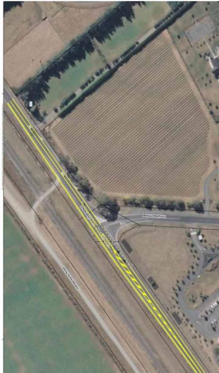
Figure 2: The proposed right hand turn bay intersection - State Highway 1 and Longbeach Road.
