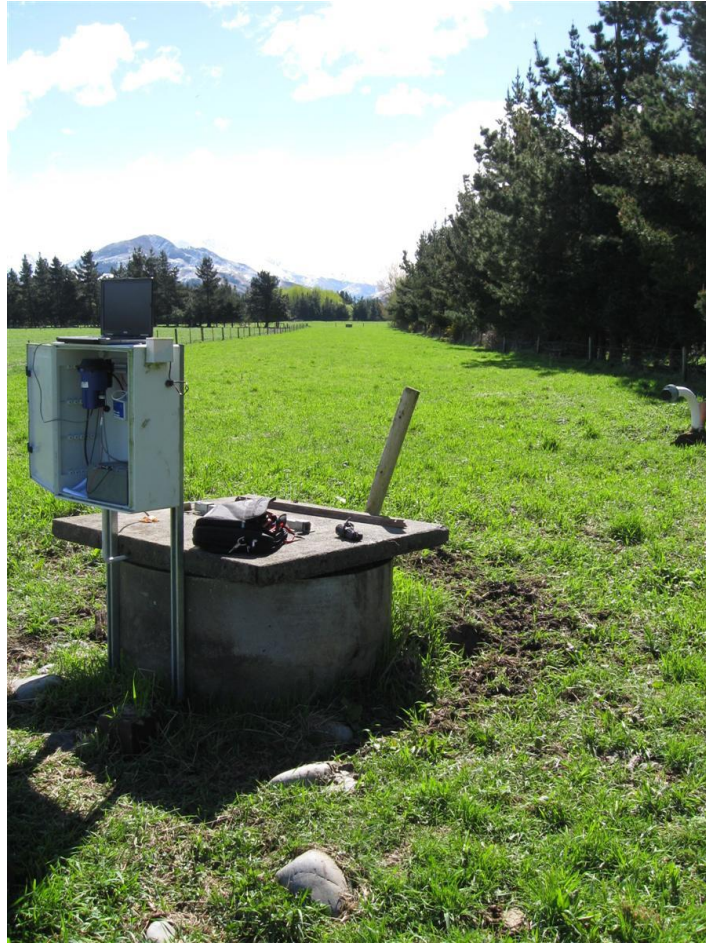
Photo 3: Supply well for infiltration gallery with monitoring equipment
