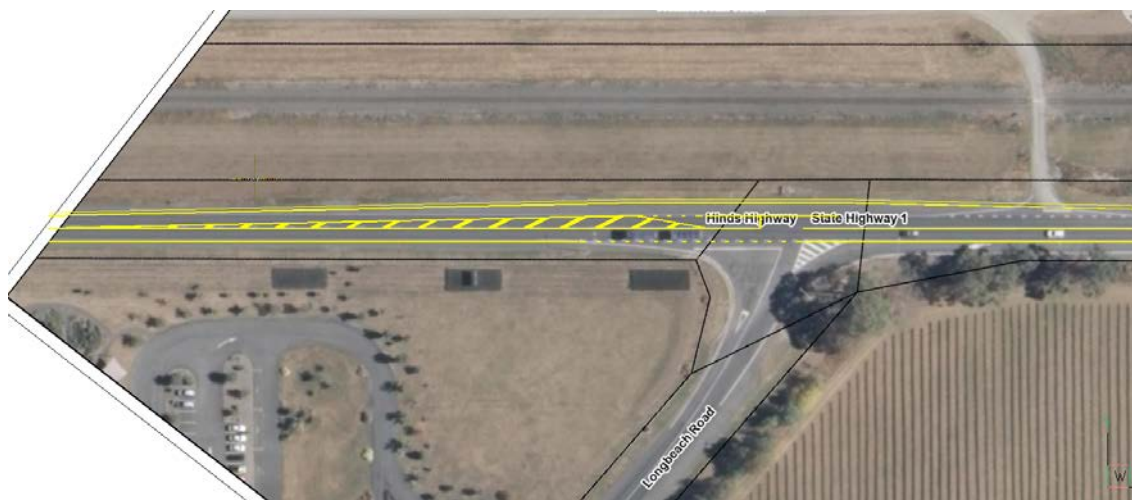
Figure 7: SH1 / Longbeach Road Right Turn Bay
